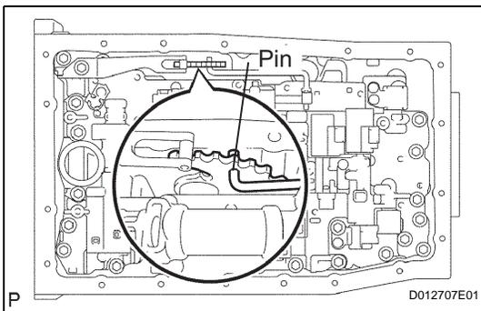
**46. INSTALL TRANSMISSION VALVE BODY ASSEMBLY**
