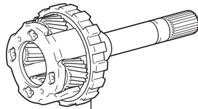
REAR PLANETARY GEAR ASSEMBLY
