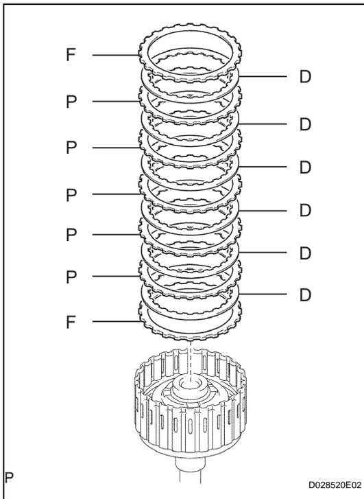
**13. INSTALL FORWARD MULTIPLE DISC CLUTCH DISC**
