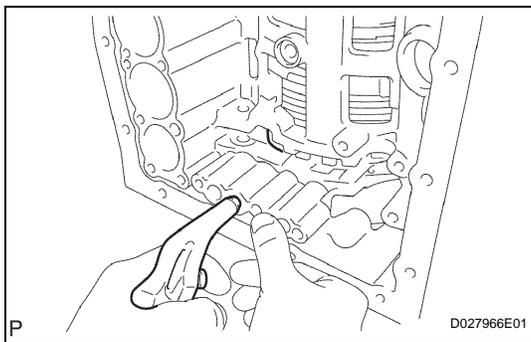
**7. INSPECT PACK CLEARANCE OF FIRST AND REVERSE BRAKE**
