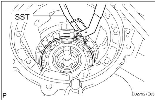
**35. REMOVE 2ND BRAKE PISTON HOLE SNAP RING**
