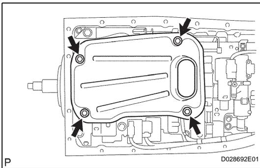
4. **REMOVE VALVE BODY OIL STRAINER ASSEMBLY**
