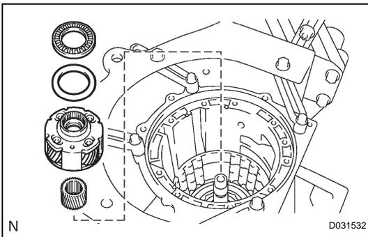
**55. REMOVE CENTER PLANETARY GEAR ASSEMBLY**
