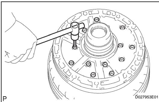
**4. REMOVE STATOR SHAFT ASSEMBLY**
