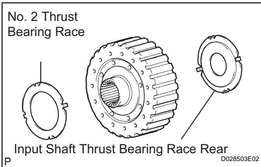
(b) Remove the No. 2 thrust bearing race and input shaft thrust bearing race rear from the multiple disc clutch hub.
