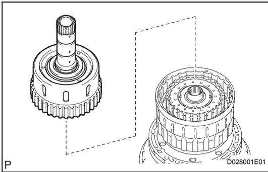
**7. REMOVE FORWARD CLUTCH HUB SUB-ASSEMBLY**
