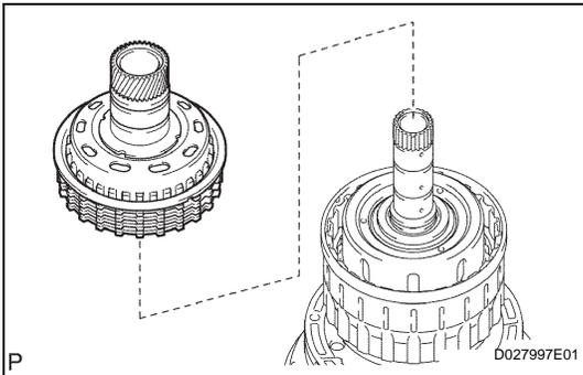
**21. INSTALL REVERSE CLUTCH HUB SUB-ASSEMBLY**
