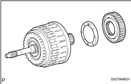
**30. INSTALL NO. 2 1-WAY CLUTCH ASSEMBLY**
