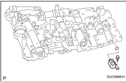
**8. REMOVE SHIFT SOLENOID VALVE S2**
