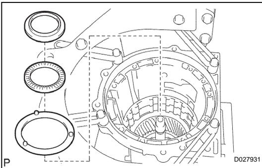
(b) Remove the thrust needle roller bearing, thrust bearing race No. 3 and planetary carrier thrust washer No. 2 from the front planetary gear.
