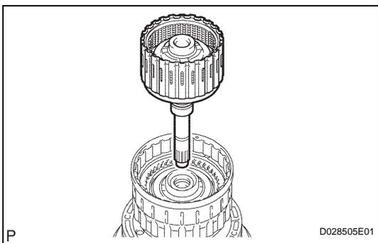
**16. INSTALL INPUT SHAFT ASSEMBLY**
