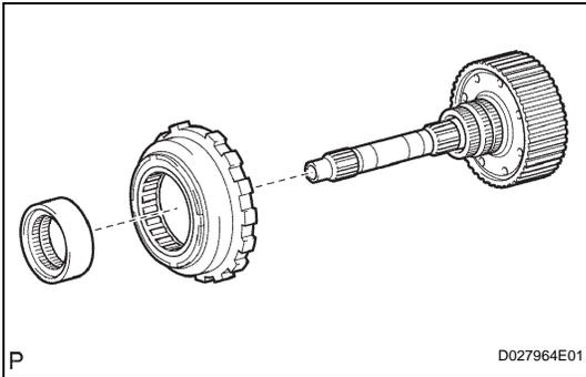
**59. REMOVE NO. 3 1-WAY CLUTCH ASSEMBLY**
