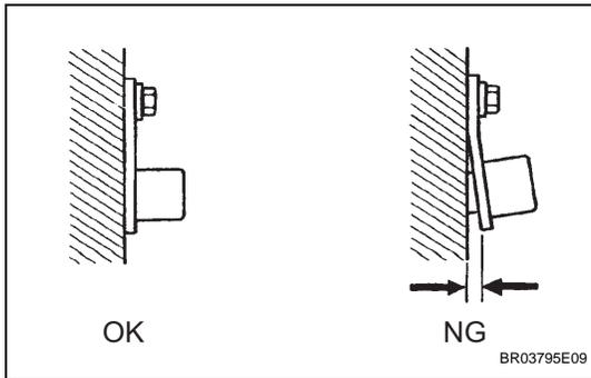
(a) Check the speed sensor (NT) installation.
