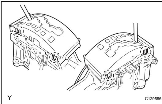
6. **INSTALL FLOOR SHIFT POSITION INDICATOR HOUSING SUB-ASSEMBLY**
