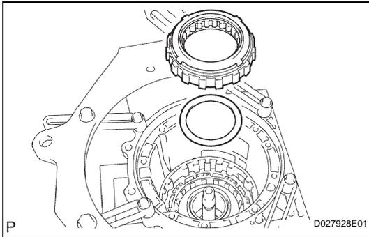
**36. REMOVE 1-WAY CLUTCH ASSEMBLY**
