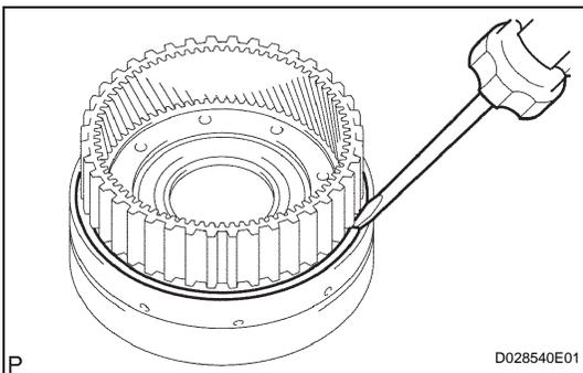
**44. REMOVE CENTER PLANETARY RING GEAR**
