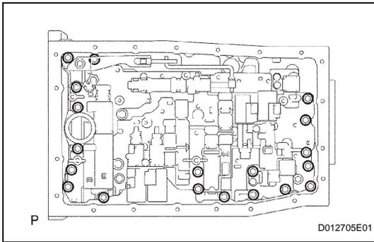
**1. REMOVE TRANSMISSION VALVE BODY ASSEMBLY**
