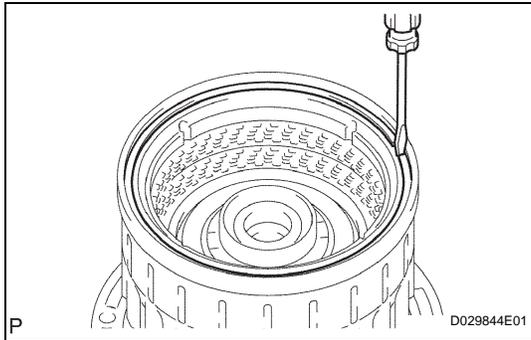
**10. REMOVE REVERSE CLUTCH REACTION SLEEVE**
