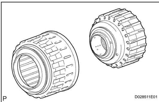
**23. REMOVE REVERSE CLUTCH PISTON SUB-ASSEMBLY**
