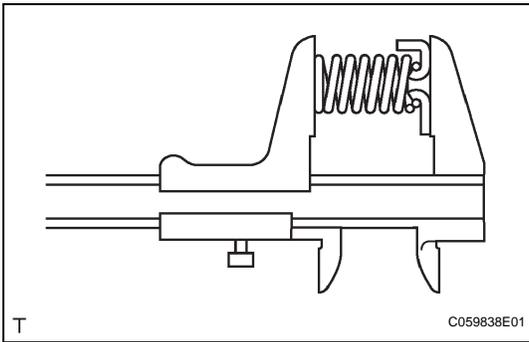
**7. INSPECT REVERSE CLUTCH RETURN SPRING SUB-ASSEMBLY**
