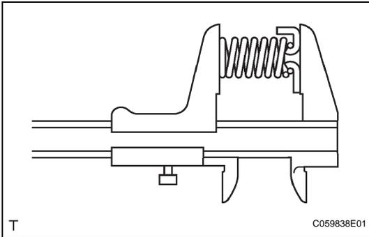
**8. INSPECT DIRECT CLUTCH RETURN SPRING SUB-ASSEMBLY**
