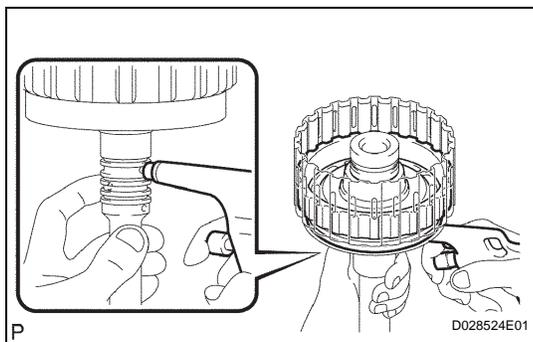
**16. REMOVE FORWARD CLUTCH PISTON**
