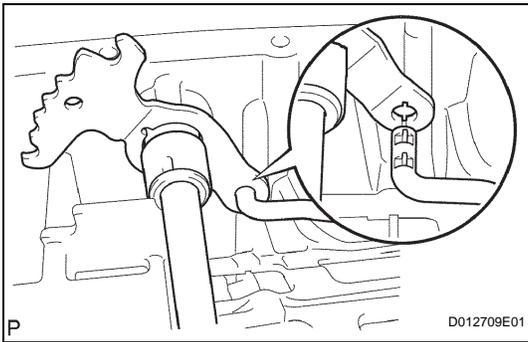
**24. REMOVE PARKING LOCK ROD SUB-ASSEMBLY**
