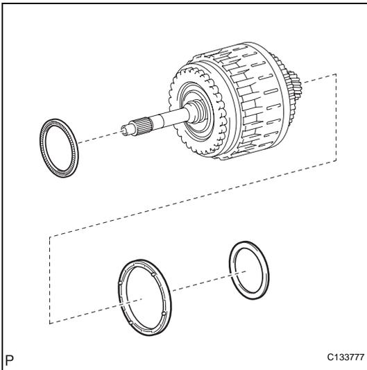
**31. INSTALL CLUTCH DRUM AND INPUT SHAFT ASSEMBLY**
