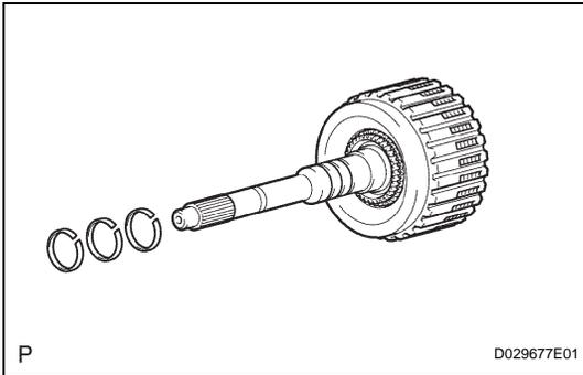
**11. REMOVE INPUT SHAFT OIL SEAL RING**
