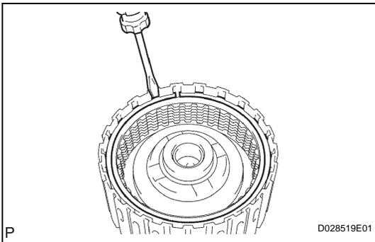
**12. REMOVE FORWARD MULTIPLE DISC CLUTCH DISC**
