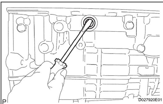
**27. REMOVE MANUAL VALVE LEVER SHAFT OIL SEAL**
