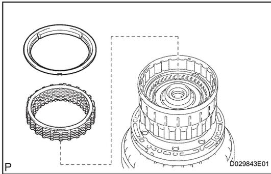
**8. INSTALL REVERSE CLUTCH REACTION SLEEVE**
