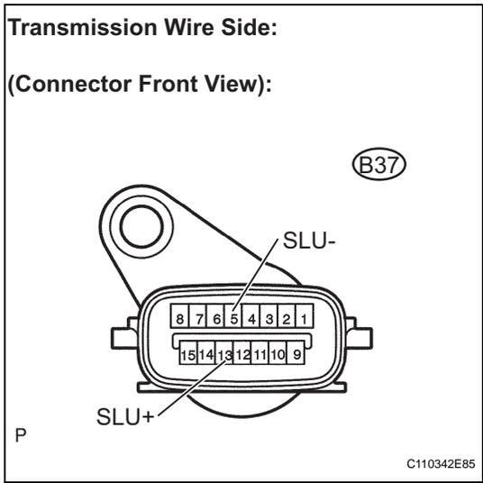
(a) Disconnect the transmission wire connector from the transmission.
