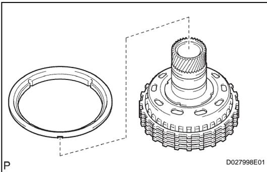
**20. INSTALL REVERSE CLUTCH REACTION SLEEVE**
