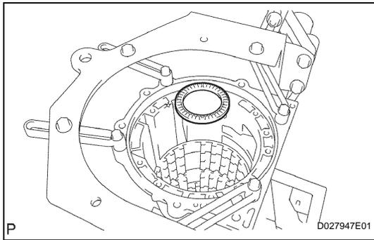
**6. INSTALL REAR PLANETARY GEAR ASSEMBLY**
