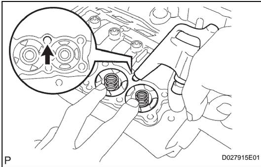
**20. REMOVE B-3 ACCUMULATOR PISTON**
