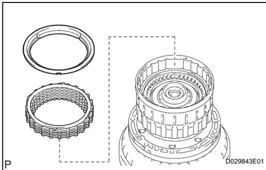
**11. INSTALL FORWARD CLUTCH PISTON**
