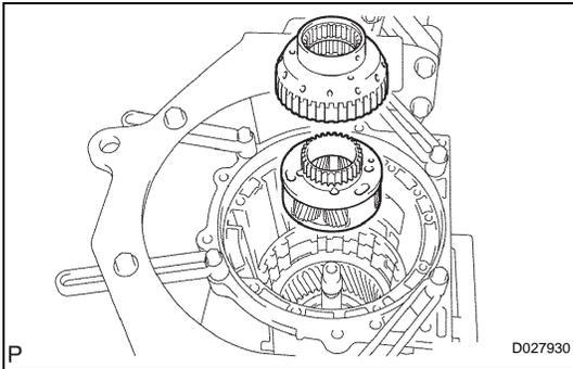
**40. REMOVE FRONT PLANETARY GEAR ASSEMBLY**
