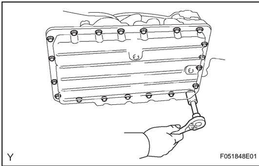
**4. INSTALL AUTOMATIC TRANSMISSION OIL PAN SUB-ASSEMBLY**
