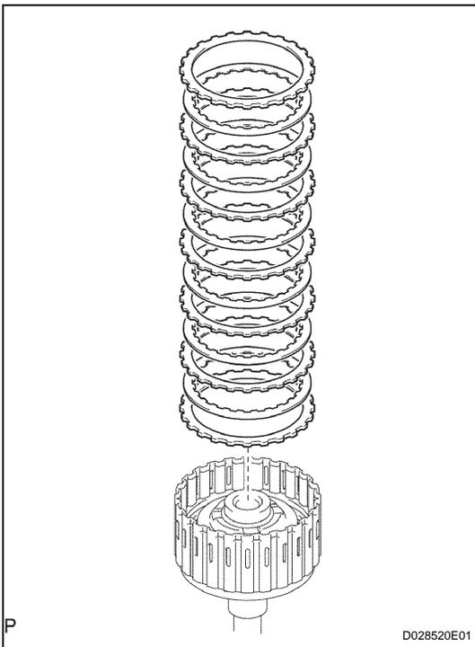
(b) Remove the 2 flanges, 6 discs and 5 plates from the input shaft assembly.
