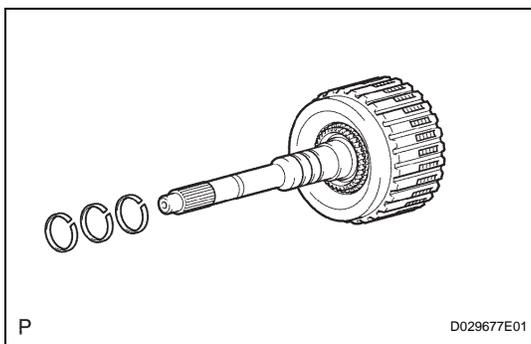
**14. INSTALL INPUT SHAFT OIL SEAL RING**
