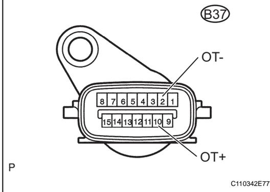
(a) Disconnect the transmission wire connector from the transmission.
