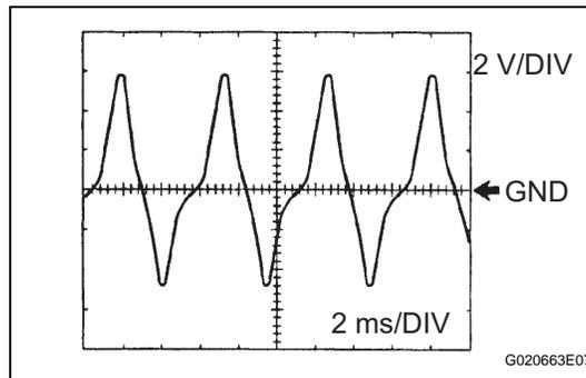
Check the waveform between terminals NT+ and NT- of the ECM connector.
