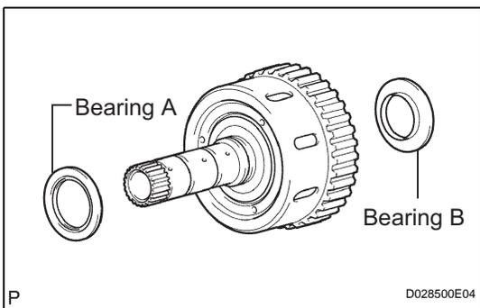
**18. INSTALL FORWARD CLUTCH HUB SUB-ASSEMBLY**
