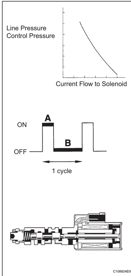
The linear solenoid valve (SLT) controls the transmission line pressure for smooth transmission operation based on signals from the throttle position sensor and the vehicle speed sensor. The ECM adjusts the duty ratio\* of the SLT solenoid valve output signal to control the hydraulic line pressure coming from the primary regulator valve. Appropriate line pressure assures smooth shifting with varying engine outputs.
