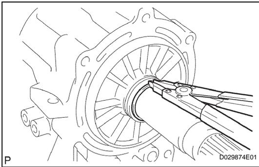
**53. INSTALL EXTENSION HOUSING SUB-ASSEMBLY**
