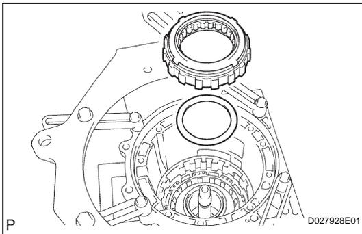
**26. INSTALL 1-WAY CLUTCH ASSEMBLY**
