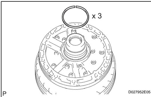
**3. REMOVE CLUTCH DRUM OIL SEAL RING**
