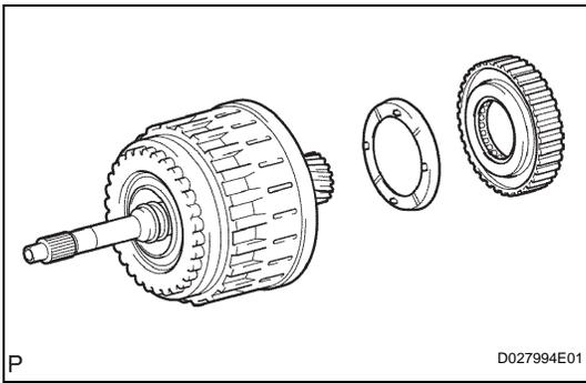
**31. REMOVE NO. 2 1-WAY CLUTCH ASSEMBLY**
