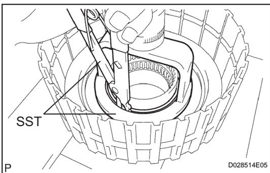
**24. REMOVE DIRECT CLUTCH PISTON SUB-ASSEMBLY**
