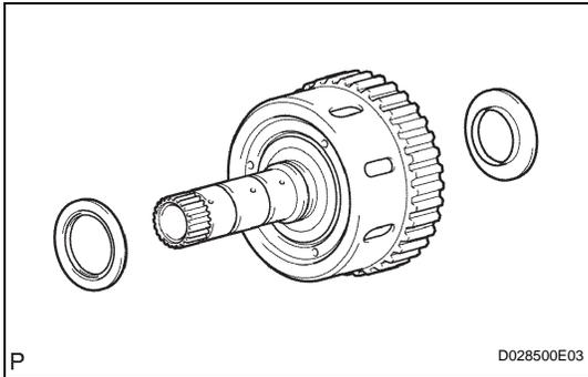
(b) Remove the 2 thrust needle roller bearings from the forward clutch hub sub-assembly.
