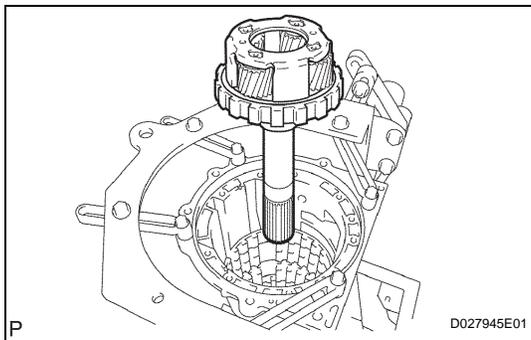
**66. REMOVE REAR PLANETARY GEAR ASSEMBLY**
