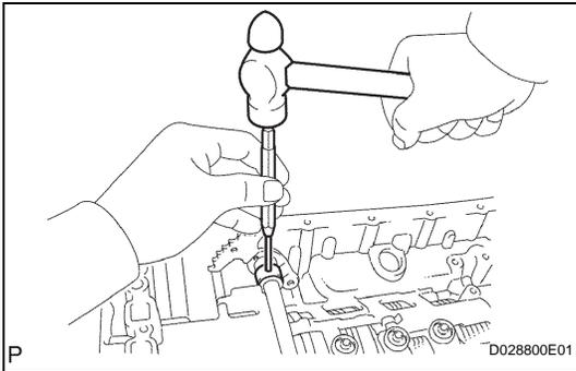
(d) Align the manual valve lever indentation with the spacer hole, and stake them together with a punch.
