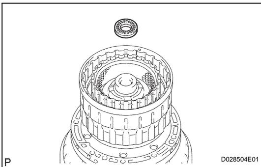
**10. REMOVE INPUT SHAFT ASSEMBLY**
