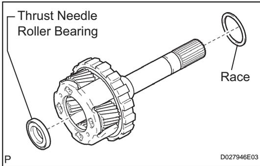
(b) Install the thrust needle roller bearing.
