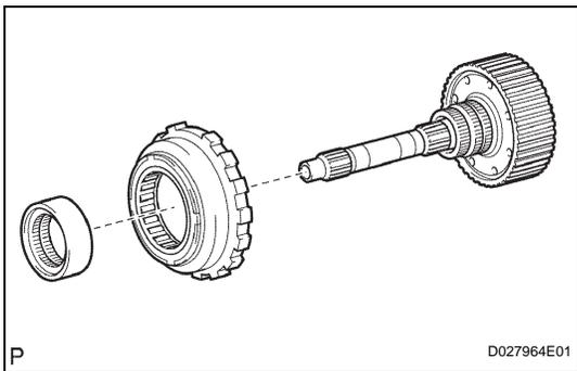
**11. INSTALL NO. 3 1-WAY CLUTCH ASSEMBLY**
