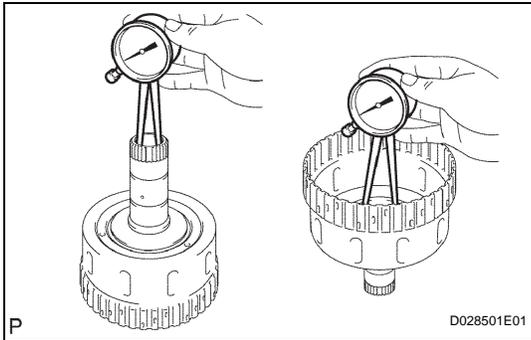
**3. INSPECT FORWARD CLUTCH HUB SUB-ASSEMBLY**
