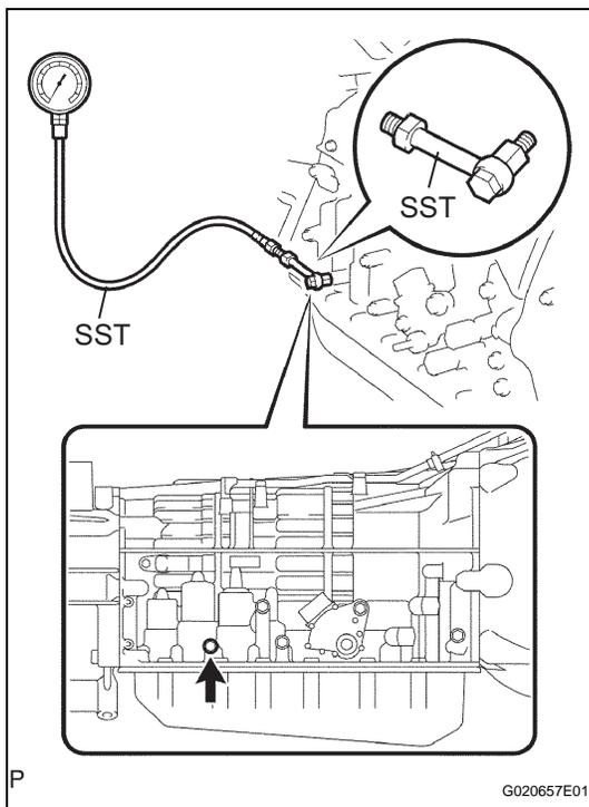
**HYDRAULIC TEST****1. PERFORM HYDRAULIC TEST**
