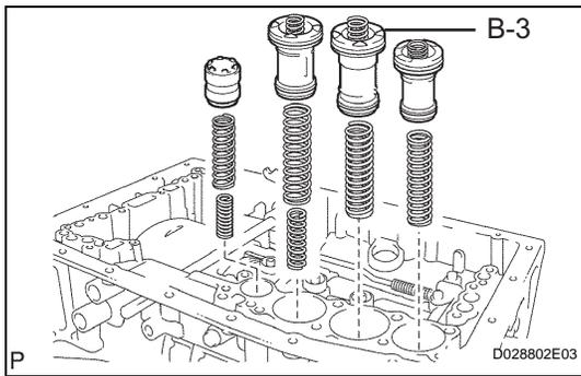
**41. INSTALL B-3 ACCUMULATOR PISTON**
