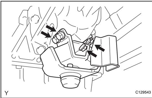
**22. REMOVE REAR NO.1 ENGINE MOUNTING INSULATOR**
