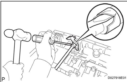
**26. REMOVE MANUAL VALVE LEVER SUB-ASSEMBLY**
