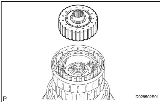
**9. REMOVE MULTIPLE DISC CLUTCH HUB**
