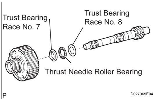
**60. REMOVE REAR PLANETARY RING GEAR FLANGE SUB-ASSEMBLY**
