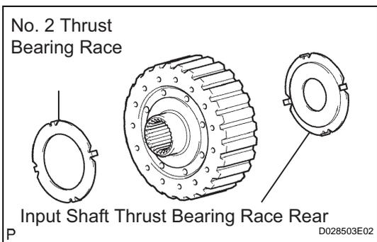
**17. INSTALL MULTIPLE DISC CLUTCH HUB**
