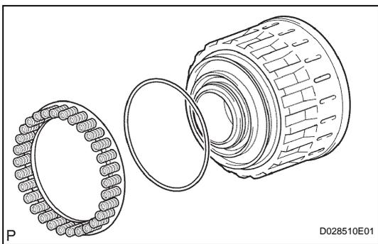
**21. REMOVE REVERSE CLUTCH RETURN SPRING SUB-ASSEMBLY**
