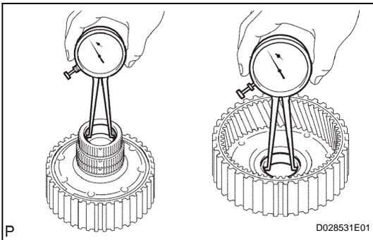
**13. INSPECT REAR PLANETARY RING GEAR FLANGE SUB-ASSEMBLY**
