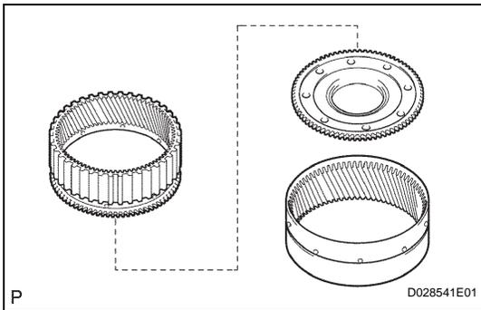
**20. INSTALL CENTER PLANETARY RING GEAR**
