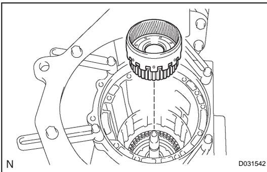
**43. REMOVE FRONT PLANETARY RING GEAR**
