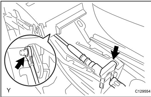
(e) Connect the control cable with a new lock clip.
