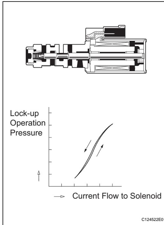
The ECM uses the signals from the throttle position sensor, mass air flow meter, turbine (input) speed sensor, output speed sensor and crankshaft position sensor, to monitor the engagement condition of the lock-up clutch.
