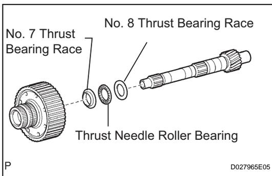
**10. INSTALL REAR PLANETARY RING GEAR FLANGE SUB-ASSEMBLY**
