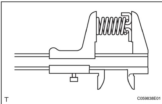
**5. INSPECT FORWARD CLUTCH RETURN SPRING SUB-ASSEMBLY**
