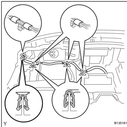
**43. REMOVE ANTENNA CORD SUB-ASSEMBLY**
