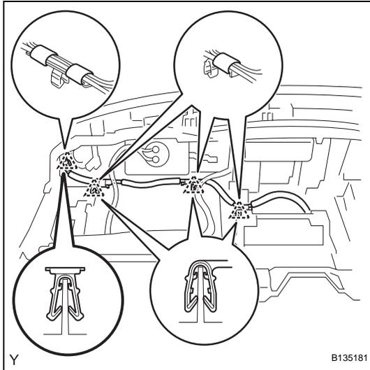
1. **INSTALL ANTENNA CORD SUB-ASSEMBLY**
