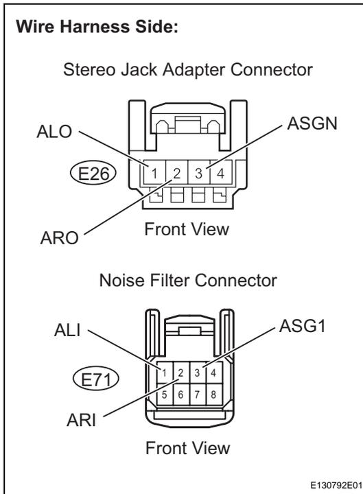
(a) Disconnect the E26 stereo jack adapter and E71 noise filter connectors.
