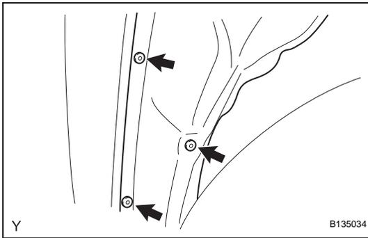
2. **INSTALL FENDER SPLASH REAR SHIELD SUB-ASSEMBLY**
