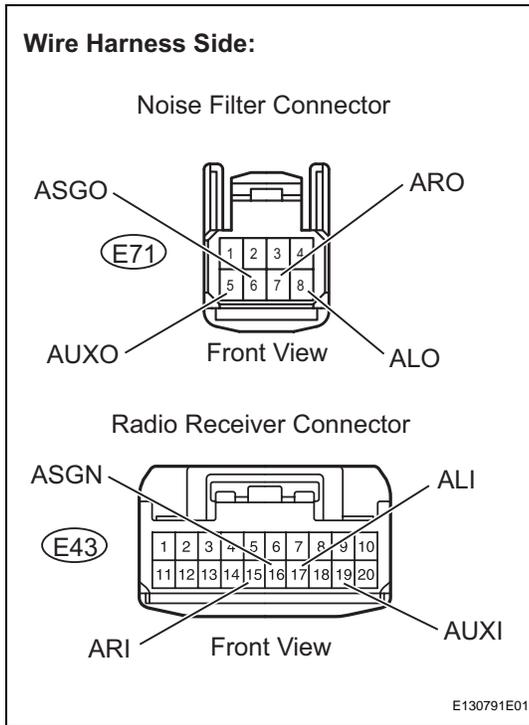
(a) Disconnect the E71 noise filter and E43 radio receiver connectors.
