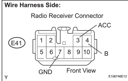
(a) Disconnect the E41 receiver connector.
