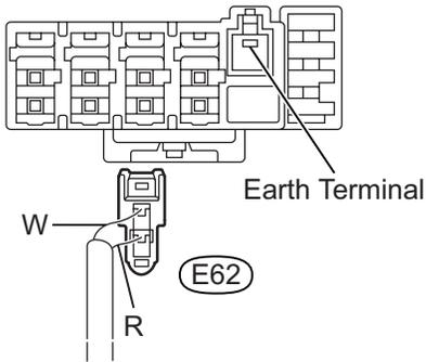
(a) Disconnect the E62 CAN main wire connector.
