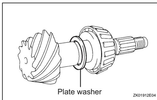
If the teeth are not engaged properly, use the following chart to select an appropriate washer for correction.
