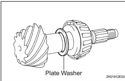
If the teeth are not engaged properly, use the following chart to select a proper washer.
