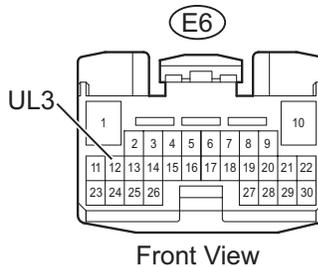
Front Door Lock Assembly LH Connector
