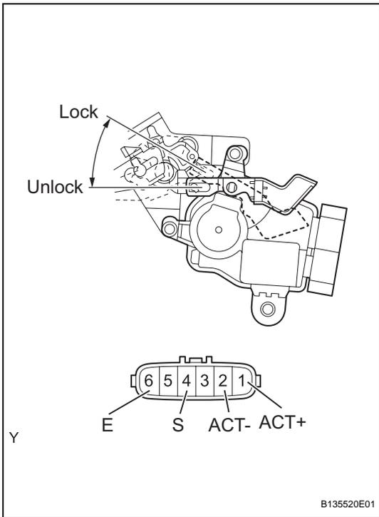
(a) Apply the battery voltage to the door lock motor and check the operation of the door lock motor.
