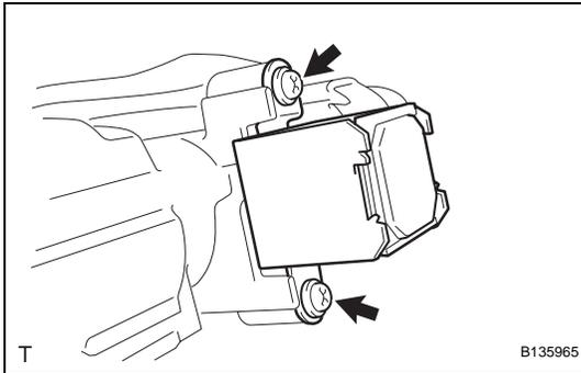
2. **INSTALL KEY INTER LOCK SOLENOID (for Automatic Transmission)**
