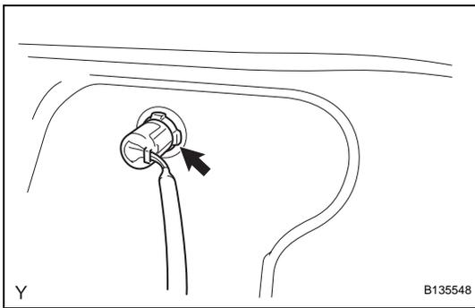
(b) Remove the back door lock cylinder.
