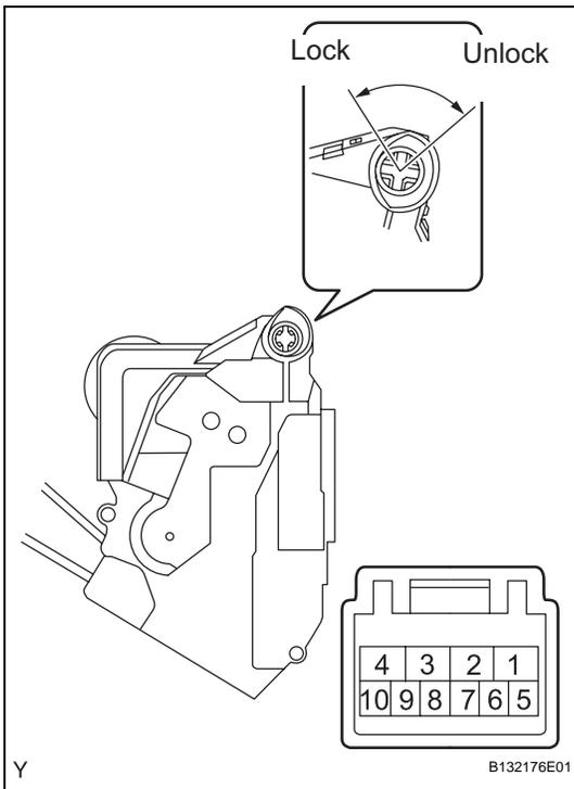
(c) Check the resistance of the door lock and unlock switch.
