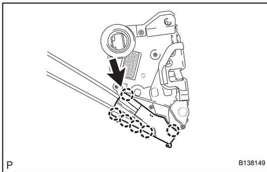
(c) Disengage the 5 claws and open the cover.
