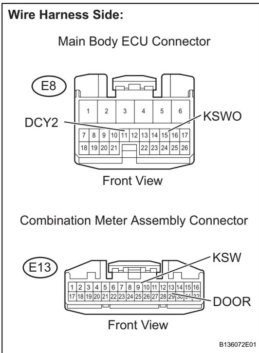
(a) Disconnect the E8 main body ECU connector.
