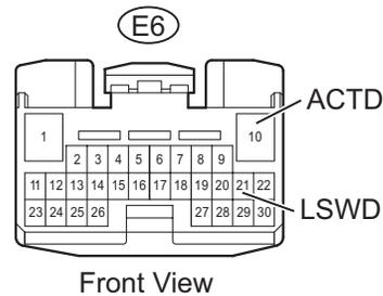
Front Door Lock Assembly LH Connector
