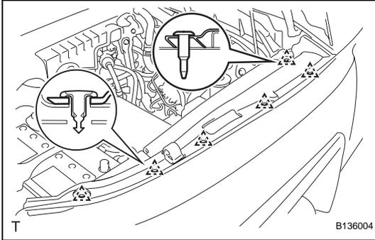
(b) Disengage the 3 clips and remove the front fender splash shield.
