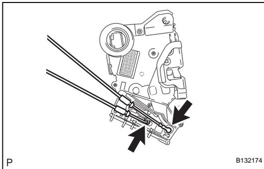
(d) Disconnect the front door lock remote control cable and the front door inside locking cable.
