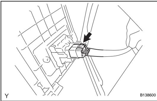
(b) Disconnect the power outlet connector.
