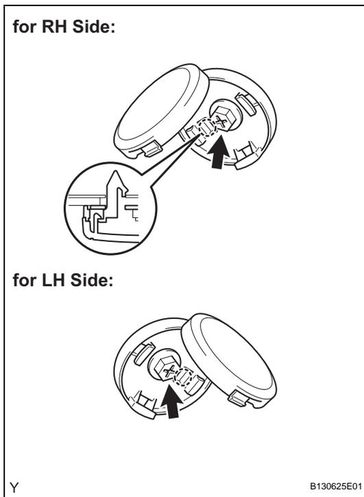
**12. INSTALL ROOF HEADLINING HOLE PLUG**
