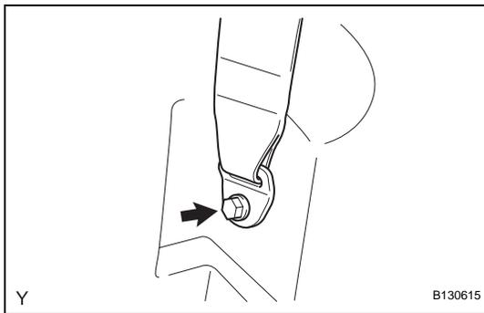
**36. REMOVE REAR SEAT OUTER BELT ASSEMBLY RH**
