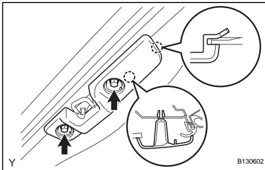
**20. REMOVE ROOF SIDE RAIL GARNISH RH**
