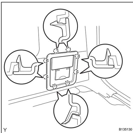
**38. REMOVE REAR DECK TRIM COVER (w/ Power Outlet Socket)**
