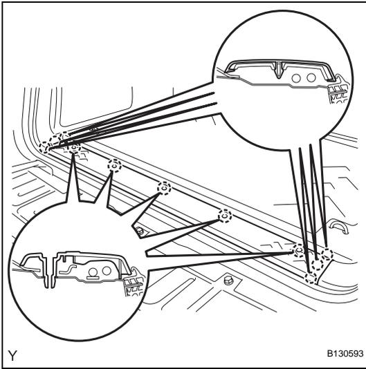
(b) Disengage the 11 claws and remove the rear floor mat support plate.
