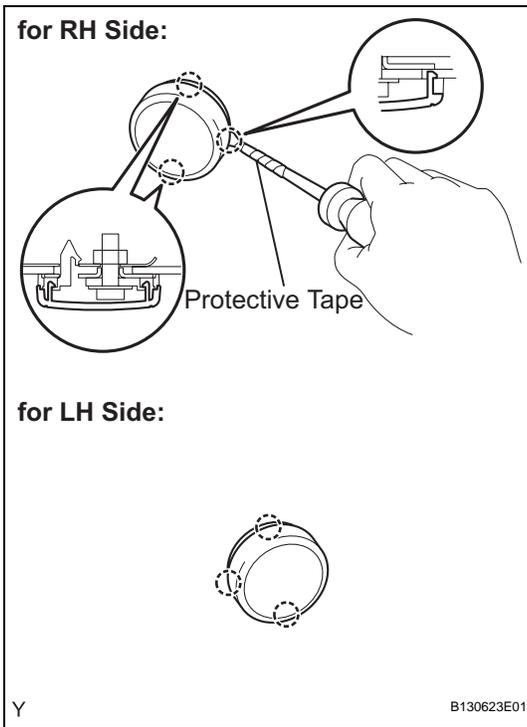
**43. REMOVE ROOF HEADLINING HOLE PLUG**
