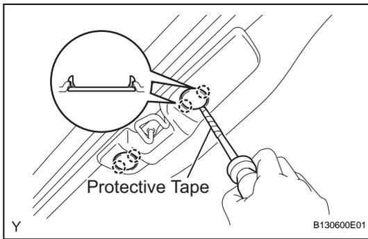
**18. REMOVE ROOF SIDE INNER GARNISH COVER RH**
