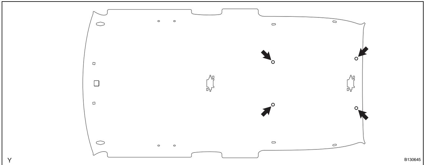
(f) Remove the roof headlining from the back door.
