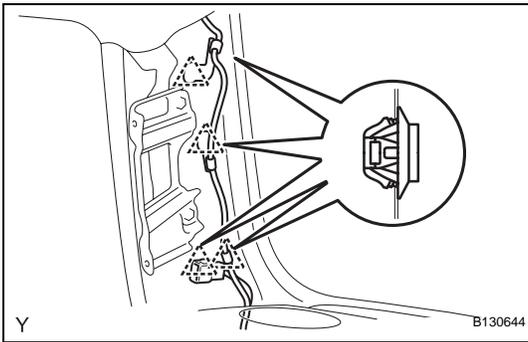
(c) Install the 3 clamps and the connector.
