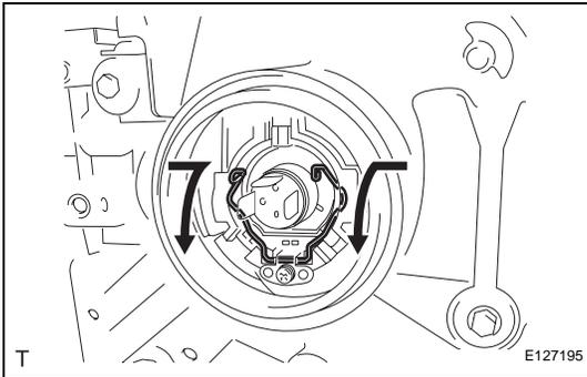
(b) Push the set spring, and pull it in the direction indicated by the arrows in the illustration, to disengage it.
