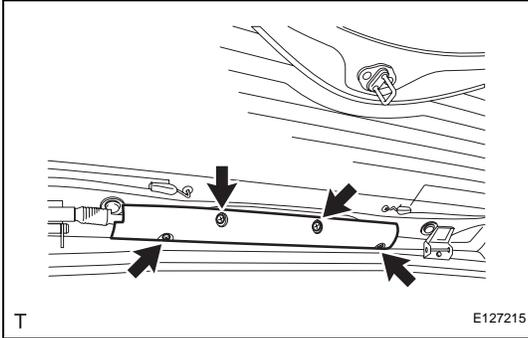
3. **REMOVE HIGH MOUNTED STOP LIGHT ASSEMBLY**
