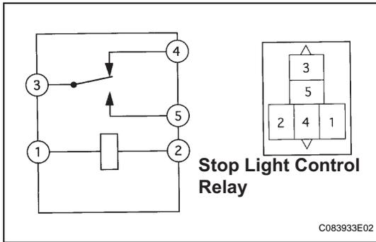
(a) Remove the STOP LP CTRL relay from the engine room R/B No. 2
