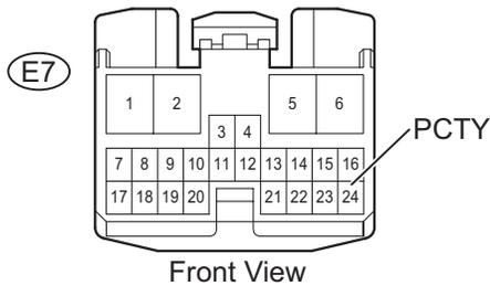
Door Courtesy Switch (Front Passenger Side) Connector
