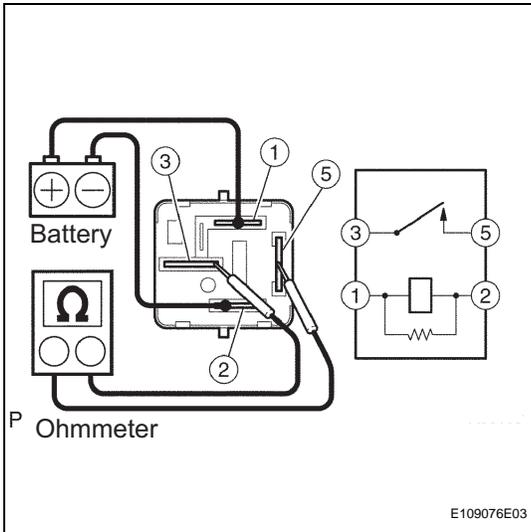
(a) Remove the DRL relay from the engine room R/B No. 4.
