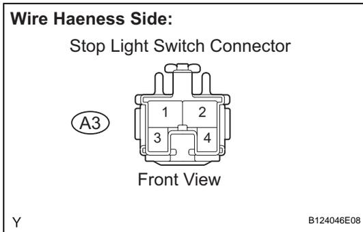
(a) Disconnect the A3 stop light switch connector.
