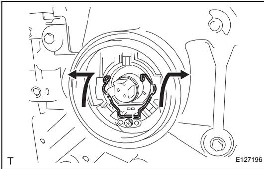
(b) Lock the set spring by moving it in the directions indicated by the arrows in the illustration.
