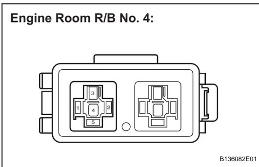
(a) Remove the DRL relay from the engine room R/B No. 4.
