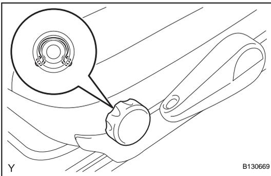
**27. INSTALL VERTICAL SEAT ADJUSTER KNOB (for Driver Side)**
