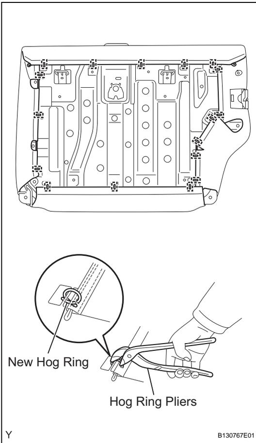
(c) Install the belt of the rear center seat outer belt into the rear seatback cover band.
