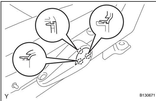
**26. INSTALL VERTICAL SEAT ADJUSTER HANDLE COVER (for Driver Side)**
