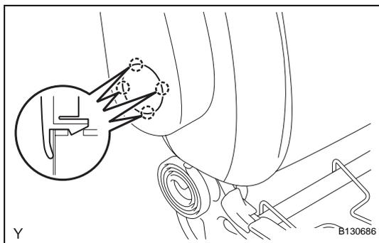
**16. INSTALL FRONT SEAT ARMREST CAP (for Driver Side)**
