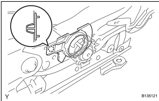
**17. REMOVE VERTICAL SEAT ADJUSTER BUSH (for Driver Side)**
