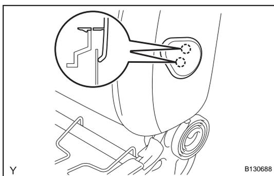
**17. INSTALL FRONT SEAT ARMREST COVER (for Front Passenger Side)**
