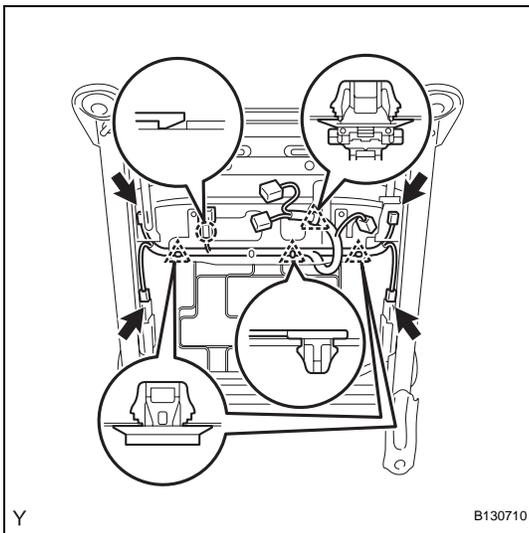
**27. REMOVE FRONT SEAT WIRE (for Front Passenger Side)**
