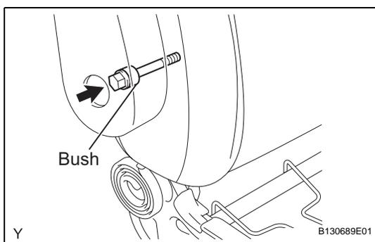
**15. INSTALL FRONT SEAT ARMREST ASSEMBLY (for Driver Side)**
