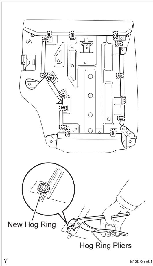
(b) Using hog ring pliers, install 14 new hog rings.
