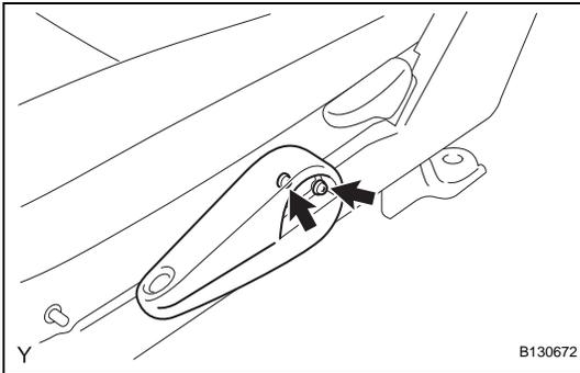
**25. INSTALL VERTICAL SEAT ADJUSTER HANDLE (for Driver Side)**
