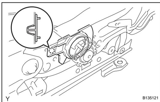
**11. INSTALL VERTICAL SEAT ADJUSTER BUSH (for Driver Side)**
